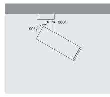
4. Adjust the angle required. Installation complete.
