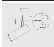
1. Unscrew to remove rotating plate from mounting base with hex wrench.
