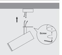
Connect wires with connector and slot into opening on mounting base, then reattach rotating plate with hex wrench.
